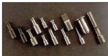
Sonotrodes adapted for different types of weld
